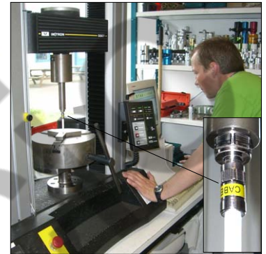
Computer controlled test of the pull strength
